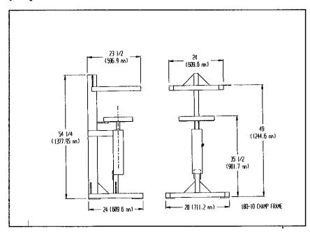
GMC 1800 CHAMP Cheese cutter for wirecuttable products up to 7" x 11" x 14". Pneumatic feed 80PSI, toggle switch speed and pressure control, unitized frame. Floor space approx. 24"x 30".
